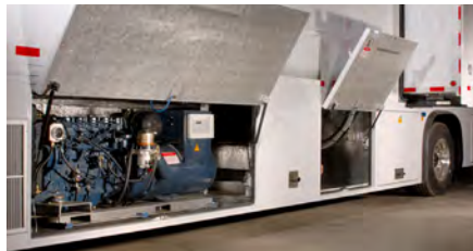
Built-In Underbelly Generator
